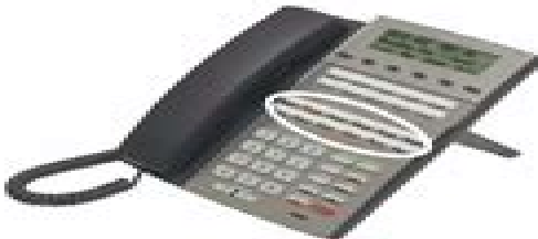
The 34-Button Display Telephone features 24 Feature Keys.
