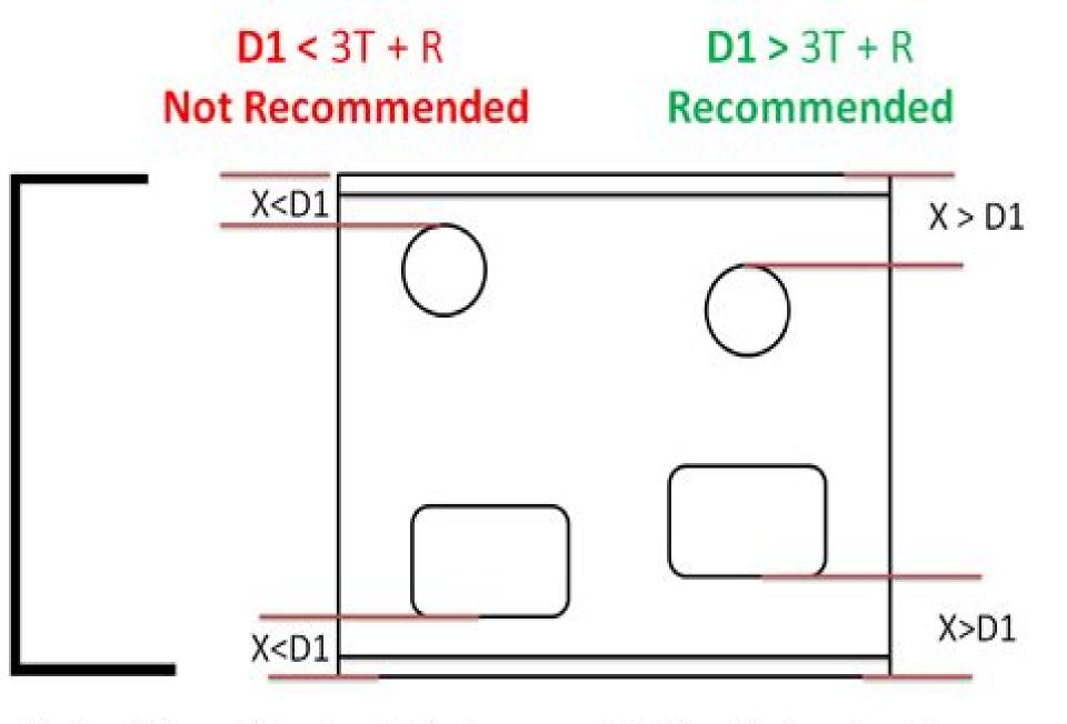
Note : Where T is sheet thickness and R is inside bend radius
