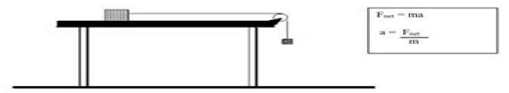
a. If the coefficient of kinetic friction, µk is 0.20., what is the acceleration of the block?  $F_n = +40N$
